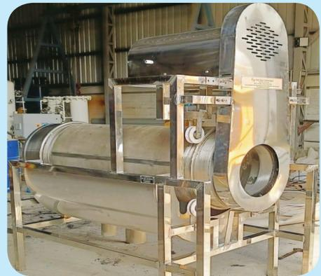
Stainless steel rotatable drum filters are used to remove the big solid particles from waste water produced by the processing industries.
