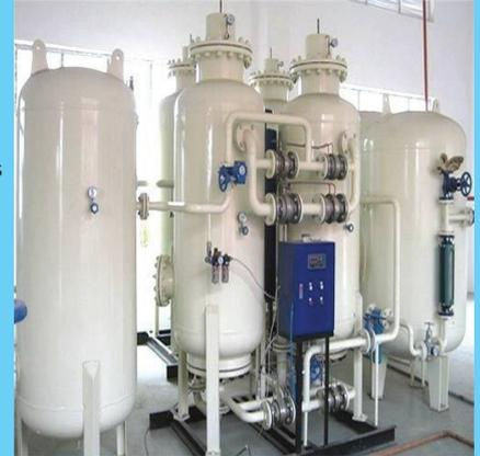
PSA type nitrogen generators are utilized extensively in food and beverage packaging, electronics manufacturing, chemical industries, medical facilities
